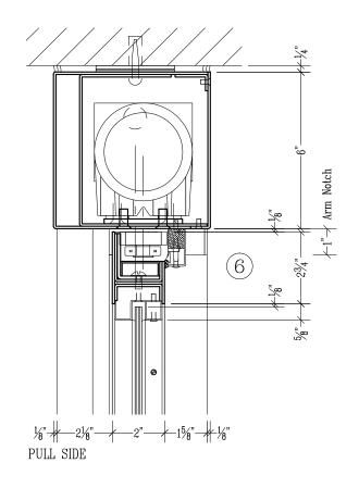
Note: Side load type power operator configurations shown at details 3 & 6 (consult factory for optional bottom load configuration if required for recessed header applications)
